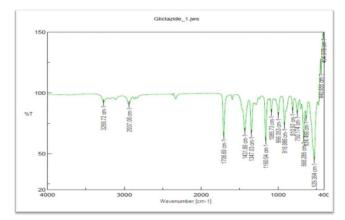
Figure 2: FT-IR Spectra of Gliclazide
